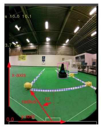
showing 1 out of 4 cameras ~100° horizontal (600px) ~135° vertical (800px) large fisheye distortion
