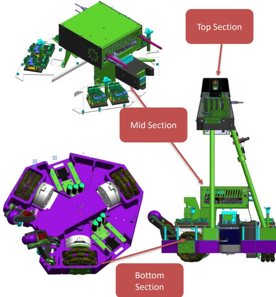
Figure 1: Robot layout in bottom, mid and top module
