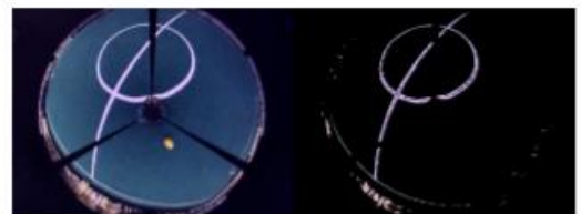
Fig. 13: Field lines are extracted using both brightness and saturation (result of step 3)
