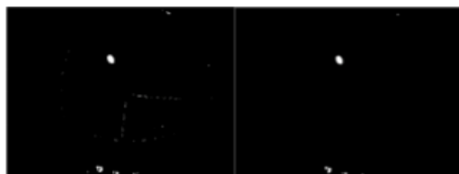
Fig. 16: Morphological filtering on the image (before in the left and after in the right)
