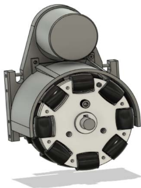
Fig. 2. Robot wheel with motor and dust cover
