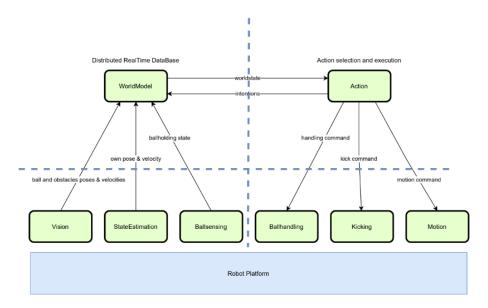
Fig. 3. Soccer Robot Architecture (Source: Eric Dortmans, Fontys)
