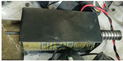
Fig. 2 Custom Solenoid attached to the bot base
