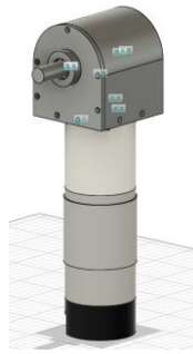
Fig. 4: Motor of active wheel with gearbox
