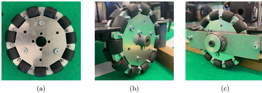
Fig. 1: Omni-Wheels: (a) One wheel assembled; (b) Wheel mounted on the robot; (c) Wheel with the outside bearing.
