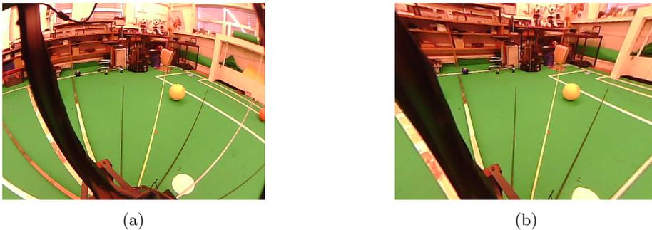
Fig. 5: Fisheye distortion: (a) Without correction; (b) With correction.
