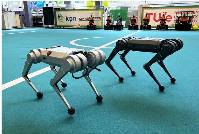
Fig. 2: MIT Mini Cheetah quadruped platforms.
