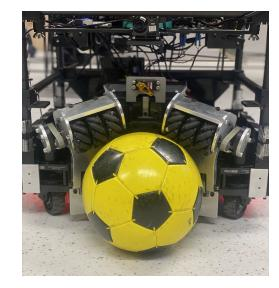
Fig. 3. Ball handling system of RCT robots
