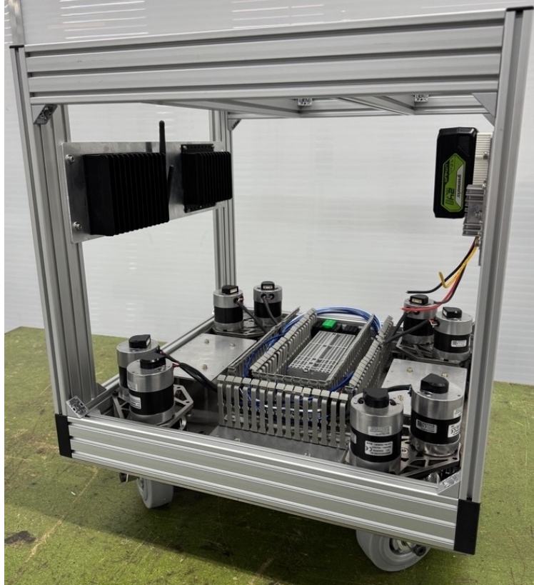
Fig. 1. Swerve drive modules with steering and propulsion motors.
