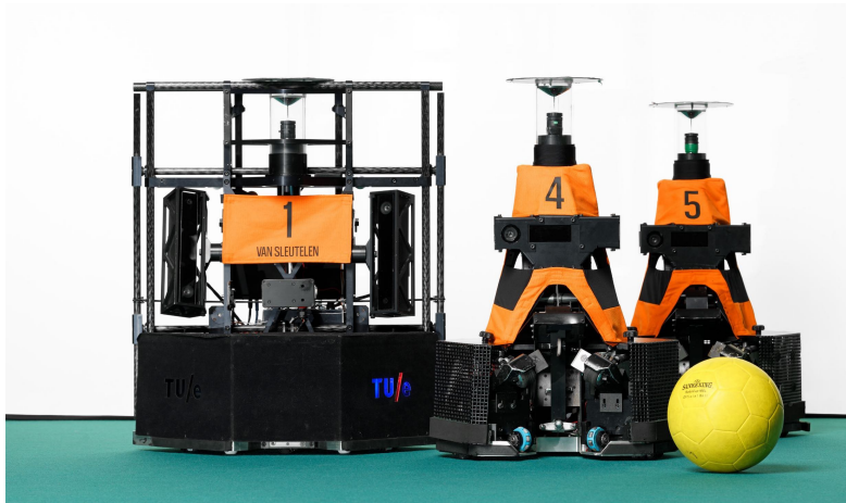
Fig. 1: Fifth generation TURTLE robots, with the goalkeeper on the left-hand side. (Photo by Bart van Overbeeke)
