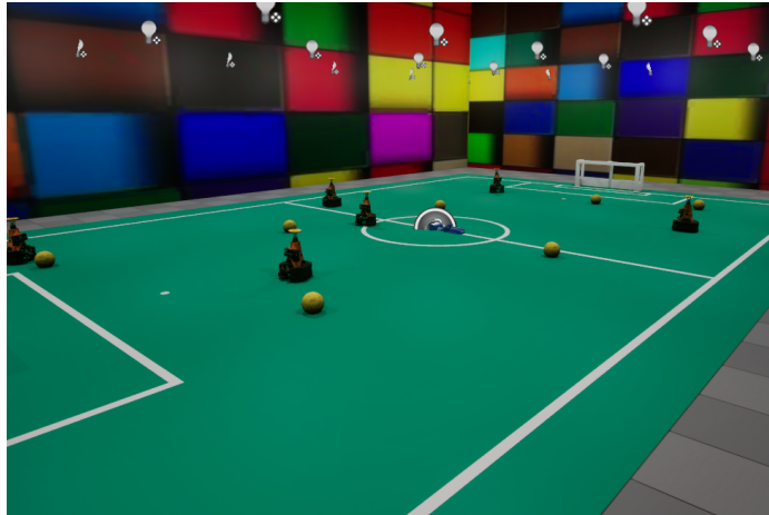
Fig. 2: Example of the virtual environment, including the field and goals, the lights, the background augmentation, and 3D Gaussian splats of balls and robots.
