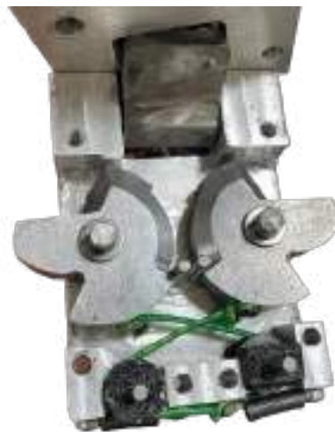
Figure 4 A "trigger" mechanism for releasing band tension with reduced force
