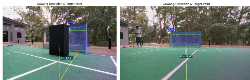
Fig. 6. Implicit Obstacle Handling. (Left) The Black obstacle naturally breaks the segmentation mask. (Right) Clear view of the goal. The algorithm dynamically discovers the largest open area (green rectangle) to establish a safe ground-level target point (red dot).
